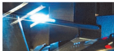
Laser equipment labels the produced tools with information on size and serial number.
